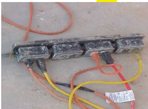
NO Homemade Power Splitters Allowed EVER, For Any Reason.
