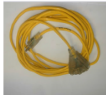
No Surge Protection
